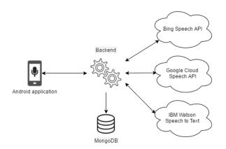
Figure 1. Architecture of the experiment
