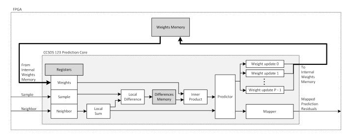
Figure 6: Compressor block diagram [4].
