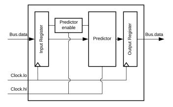
Figure 7: Predictor Co-processor Wrapper.
