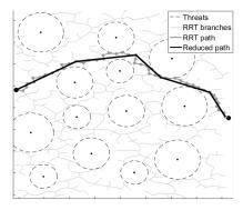
Figure 5. The RRT path planning operation.
