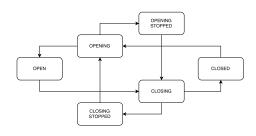
Figure 3. State diagram for the electronic gate
