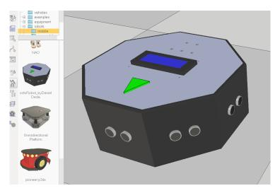
Figura 2. OCTO robot model in virtual platform V-REP.
