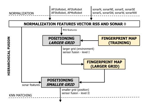
Figura 5. Hierarchical fusion block diagram, based on kNN matching algorithm.
