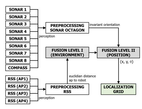
Figura 3. Hierarchical sensor fusion method block diagram.
