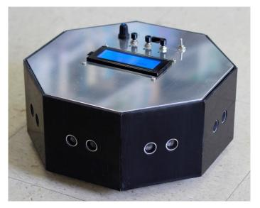
Figura 1. Mobile robot platform - OCTO robot by Daniel Deda [Magrin and Deda 2016].
