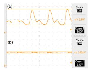
Figura 4. Signals from finger with infrared (above) and red LED (bellow).
