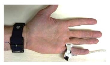
Figura 1. Arrangement of the PPG sensors to measure PTT.
