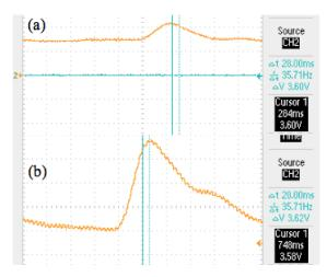
Figura 5. E-mail Peak on the wrist signal triggers the timer (above), while a peak on the finger signal stops the timer (bellow).
