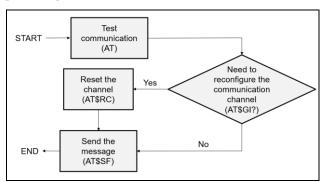
Figure 4. Process of transmission via Sigfox
