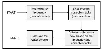
Figure 3. Process of conversion pulses into water volume
