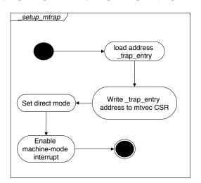
Figure 5: State diagram of the trap setup
