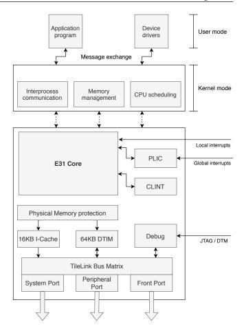
Figure 4: The microkernel and the HiFive1 board overview
