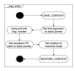
Figure 6: State diagram of the trap entry
